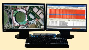
of an electrified enclosure (mimic screen) and the ease of operation that a Windows compatible GUI application can provide. It can also be integrated into existing systems using RS232, RS485 and Fibre Communication protocols.
