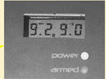
LCD ENERGISER OUT AND RETURN VOLTAGE DISPLAY
